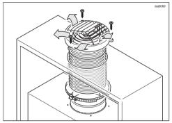
Conversion kit DUU 150 with a plastic grille is suitable for fitting in a non-visible area of the top of the wall unit.
